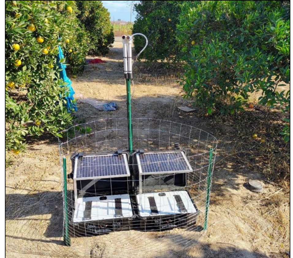
Pesticide Monitoring Equipment Setup within Fresno
