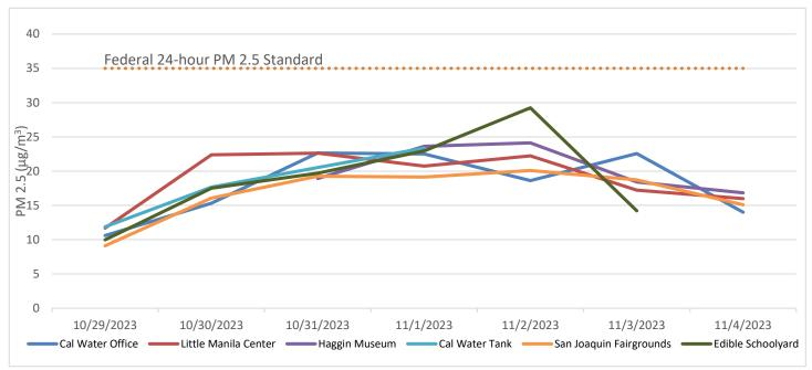
\*PM2.5 at Haggin Museum was down due to annual instrument calibration from 10/29 - 10/31 \*PM2.5 at Cal Water Tank was down due to annual instrument calibration from 11/2 - 11/4 \*PM2.5 at Edilble Schoolard was down on 11/4 due to an instrument error
