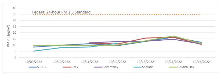
$<sup>\</sup>star$ DMV down 10/09 to 10/10 and Sequoia down 10/13 to 10/15 for calibration. Grimmway down 10/09 to 10/10 for maintenance.
